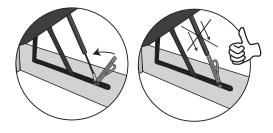
Put the plastic stopper to the gas spring so that the bed box can't close
